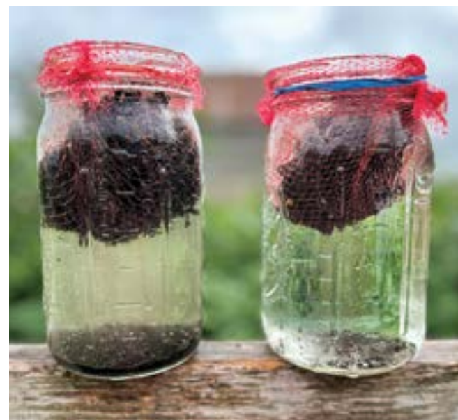
Figure 2. Comparison of two soil samples using the slake test. Less soil moved into solution with the healthier sample on the right. Soil with less structure on the left, more easily dissolved into solution and settled out to bottom of jar.
