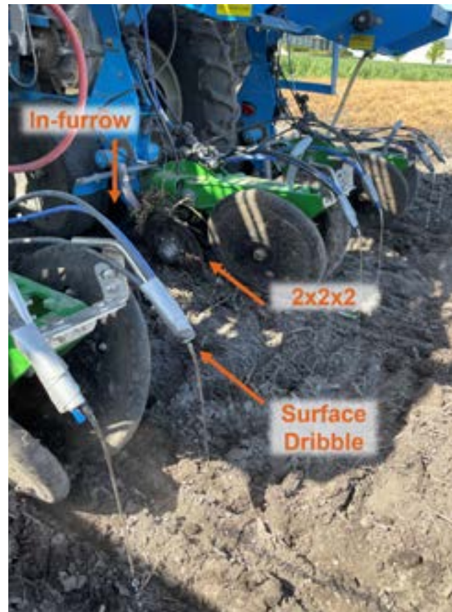
Figure 1. Planter used to apply fertilizer in-furrow, 2x2x2 and surface dribble.
