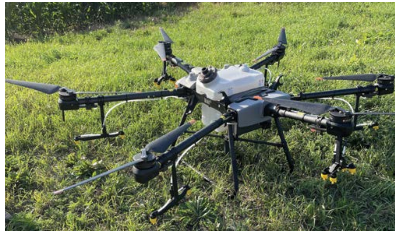
Figure 2. Example of a boomless spray drone.
