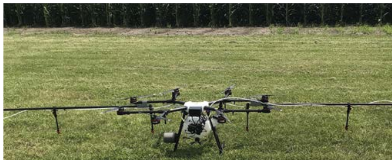
Figure 1. Example of a boomed spray drone equipped with flat fan nozzles.
