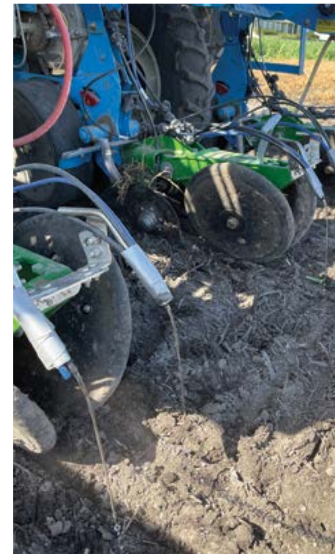
Figure 1. Planter surface dribbling nitrogen in a dual band, on either side of the seed furrow.
