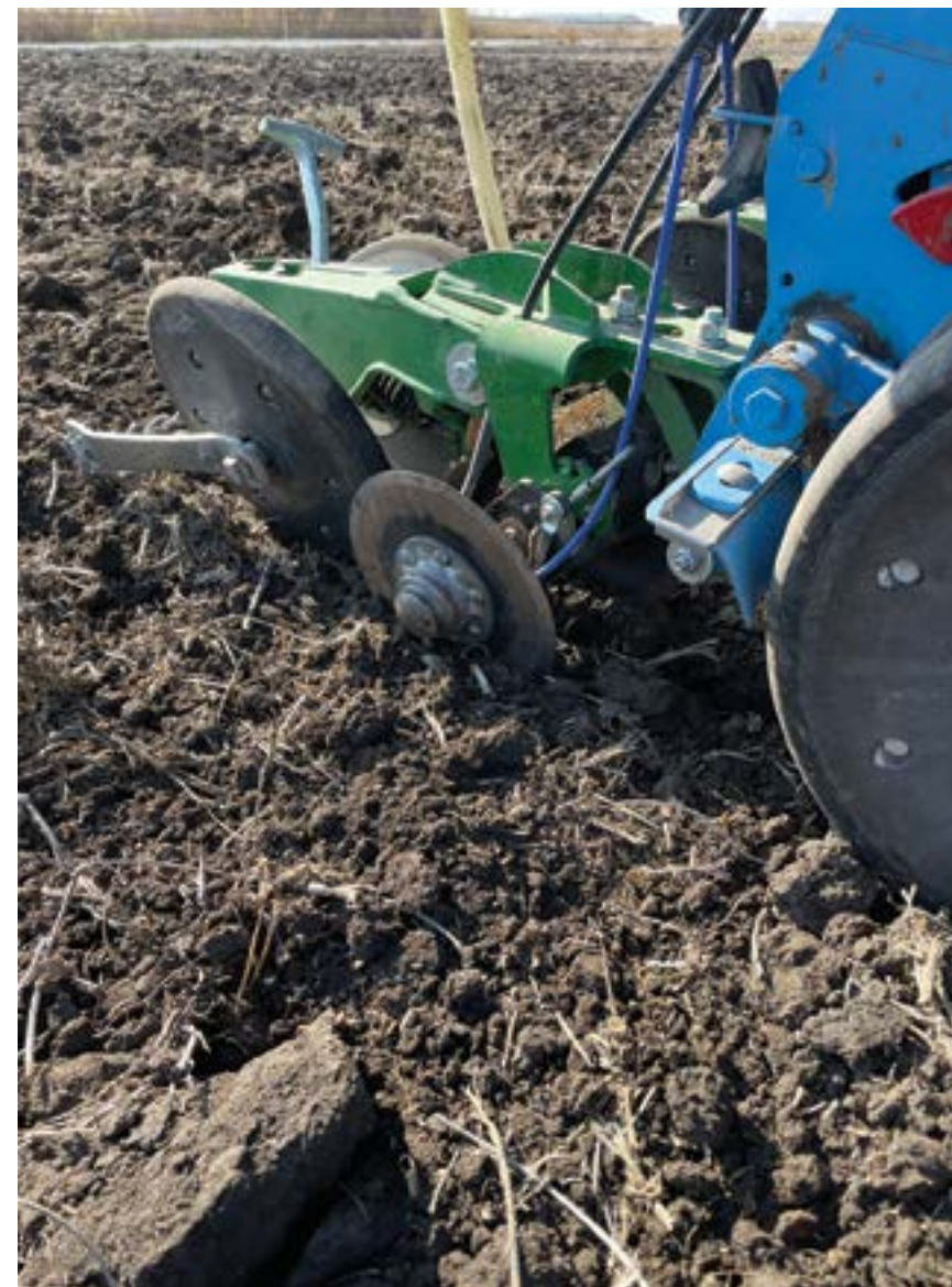
Figure 1. ATS and KTS applied with liquid fertilizer banding attachment on planter.
