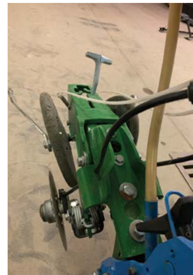
Figure 2. Planter attachment showing the 2x2x2 (dual banded, soil incorporated) nitrogen application method.
